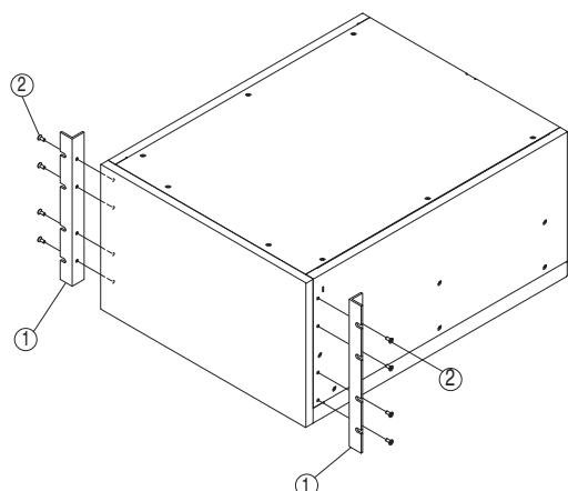
3. Using the accompanying screws and washers, mount the instrument in the rack.
