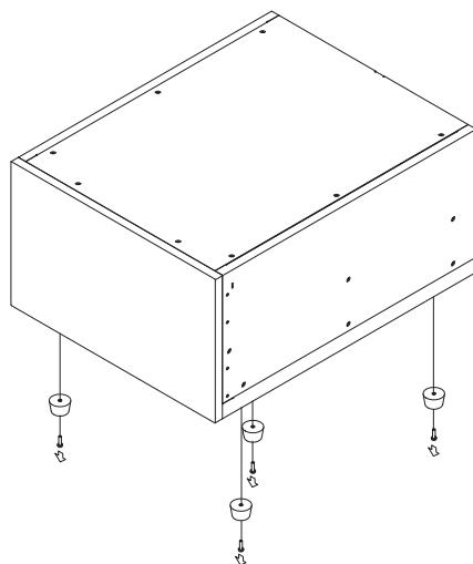
2. As shown in figure, using the accompanying screws, install the brackets. Do not use except the accompanying screws (M4 x 10 flat head screws).
